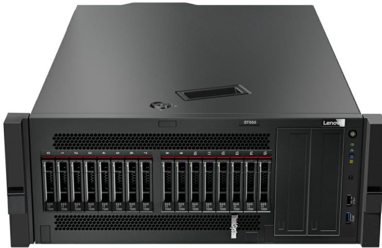
Figure 20. ThinkSystem ST550 with Rack Conversion Kit installed
